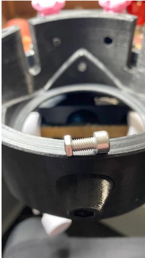
Half Nut on 12mm long M5 cap screw
