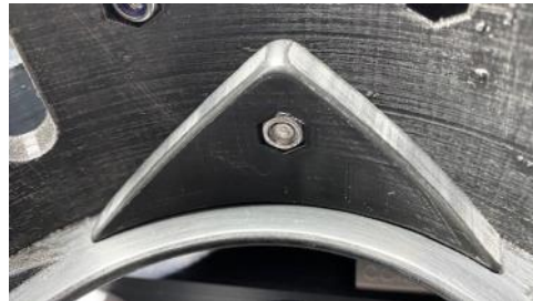
Riser Cam fastened to the inside of the casing
