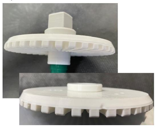
Solvent weld the dial to the bearing cover, this traps the bearing, which should have zero axial movement in the assembly. Set aside to dry after checking the rotation is wobble free by putting the assembly onto the assembly jig (with the '1' engraved on the sides) held vertically in a vice. Fit an M5 full nut to the spacer with the grooves in the side and put the dial over the screw onto the cage and spin the dial, making sure the dial rotates flat with no vertical wobble.
