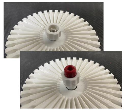
Finally, polish the front edge of the fin and attach the fin to the bottom of the dial using 2 off 3.5 x 9.5 self tapping screws, the fin can be adjusted to set the 'timing' of the ribber needles with the cylinder needles. Setting the dial timing is covered in the Ribber User Guide.
