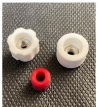
3 parts of the dial spacer, with top and knurled spacer fitted with nuts. The socket for the nut is tapered so that the nuts will be retained if you pull them in TIGHT.
