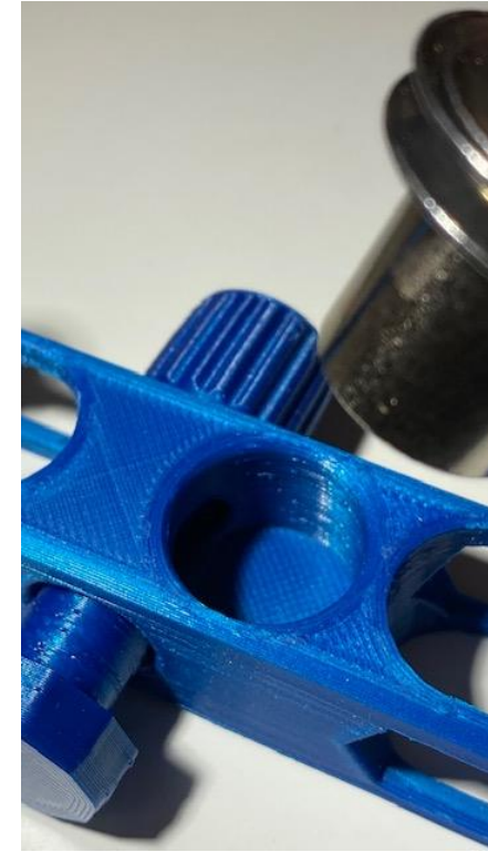
Grip Screw and nut aligned for insertion of the parallel cylinder on the back of the Tension Unit
