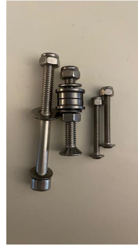
Pinion fixings – left to right: Handle bolt Pinion screw, bearings and nuts Handle screws
