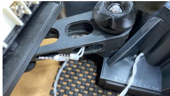
Cable routing from the bracket to the counter
