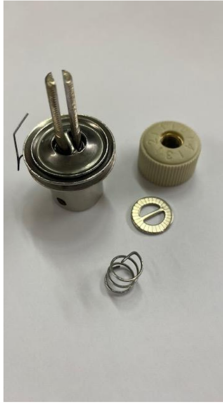
Replace Conical Spring with 8mm diameter spring made from 0.8mm wire, four turns with end 6mm bent at 90 degrees to prevent rotation at each end of the spring.
