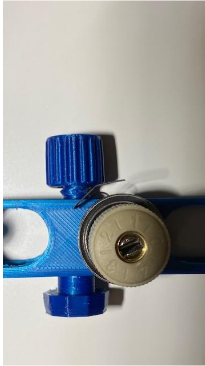
Grip Screw and Nut with Tension Unit, grip screw pushed up to engage on the tension unit, before tightening the nut.
