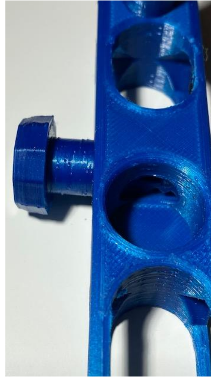
Grip Screw inserted into through hole in the parallel arm, the 'scoop' is aligned with the socket for the Tension Unit
