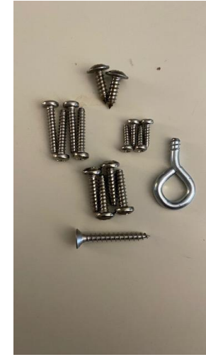
Self tapping screws from top clockwise: Counter Carrier Pivot Counter Switch and Counter Screw eye for Caston Bonnet countersunk screw for bracket spigot Cylinder screws Cam lift system screws
