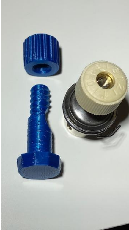
Grip Screw and Nut with Tension Unit, note 'scoop' from Grip Screw
