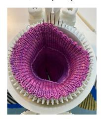
4 - Thread your waste yarn through the tension unit and feeder and around the needle at the centre uplift cam, with the yarn from the feeder **above** the latch on **every** needle.
