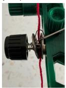
If the tension regulator is too tight, it will prevent the needle latches from opening.
