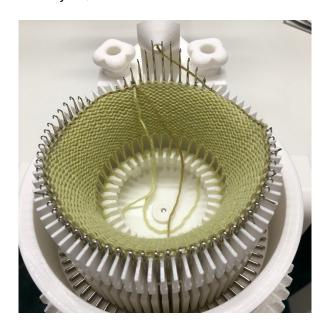
12 - Both of the yarn ends should be inside the cylinder, with the project yarn being fed from the yarn feeder.
