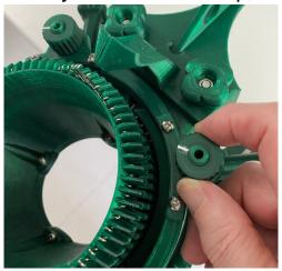
After the CAM screws have been replaced and the **CAM lock screw is still loose**
