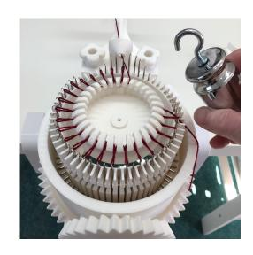
8 - The first stitches of row 1 are knit at the same time as casting on is finishing.
