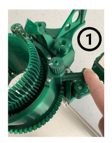
1 - Release/loosen the long **CAM lock knobs** on the back of the machine.
