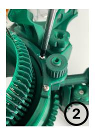
2 -Using the screwdriver provided, unscrew the screws positioned either side of the **CAM adjustment knobs.**
