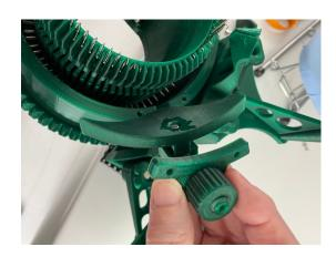
The height of both V cams can be adjusted by turning the
