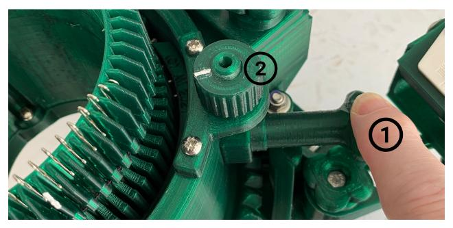
Stitches that are too tight when the needle rises towards the centre uplift CAM, will NOT drop off the needle shaft, preventing the latch from opening and creating a stitch.
