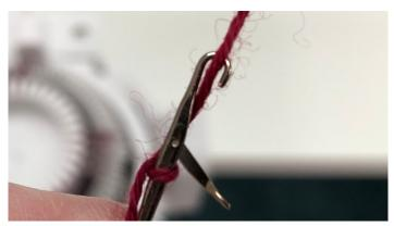
The latch on the needle does the knitting, so when the needle reaches the 2nd cam on the right hand side, the latch will close and create a stitch.
