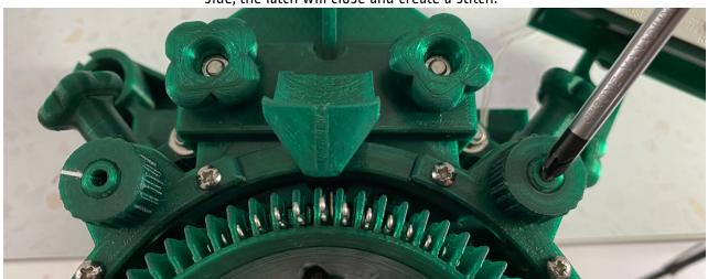
Lowering the CAMS will loosen and lengthen the stitch. Raising the CAMS will shorten and tighten the stitch.
